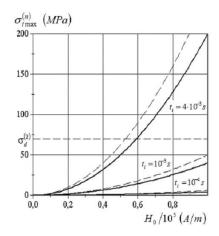
Figure 5 Dependence of the maximal values of  $\sigma_{i \max}^{(n)}$  on values of  $H_0$  for different pulse durations
