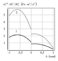
Figure 4 The plate thickness distribution of  $\sigma_i^{(n)}$  stresses intensity at different moments for duration of action in MPMS  $t_i = 100 \ \mu s$
